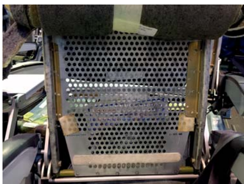
ATR SEAT CRACK REPAIR
